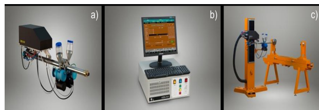
a) working body (gun), consisting of a barrel, a gas distribution block and powder dispensers; b) block control based on an industrial computer; c) gun complete with three coordinates manipulator Figure 1 – Detonation complex CCDS2000
